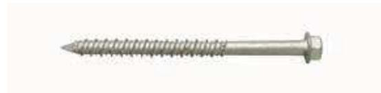
For use with 5" (12.7 cm) and higher FOUNDATION Platform Kits, these corrosion resistant 3.25" (8.26 cm) concrete anchor screws keep platforms firmly in place. Prior to installing the tiles, use a 3/16" (5mm) bit to drill 2" (5 cm) deep and secure 1 screw (bag of 10) into each leg cross brace.
