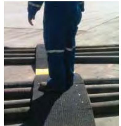
Grit Top Walking Surfaces fit on a Standard Bridge
