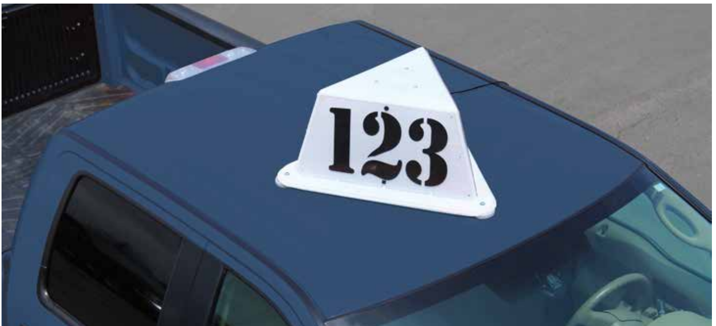
Small Vehicle Identification Light on the top of a pickup truck.
