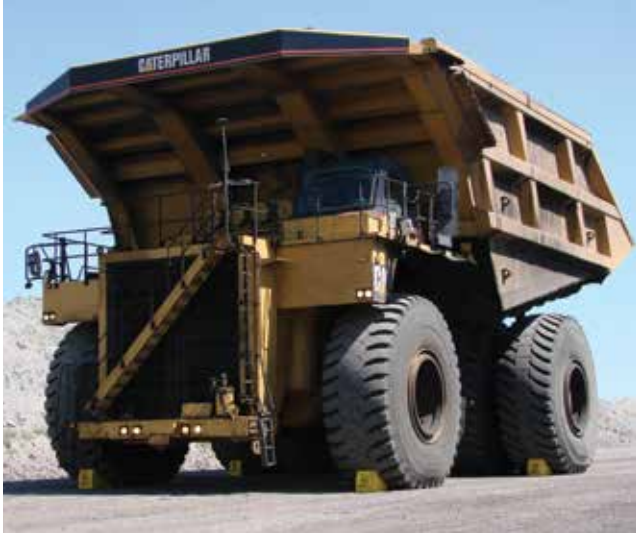
Four Monster wheel chocks, model MC3011 used on CAT 797
