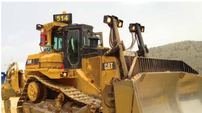
Triangular Vehicle Identification Light on a dozer.
