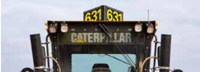
Triangular Vehicle Identification Light on a road maintenance vehicle.
